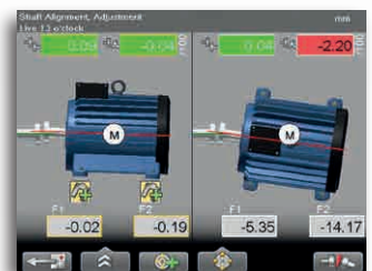
Shaft alignment program. Note! Accessories required.
